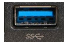
fig. 2. Examples of a USB-3.0 port.
