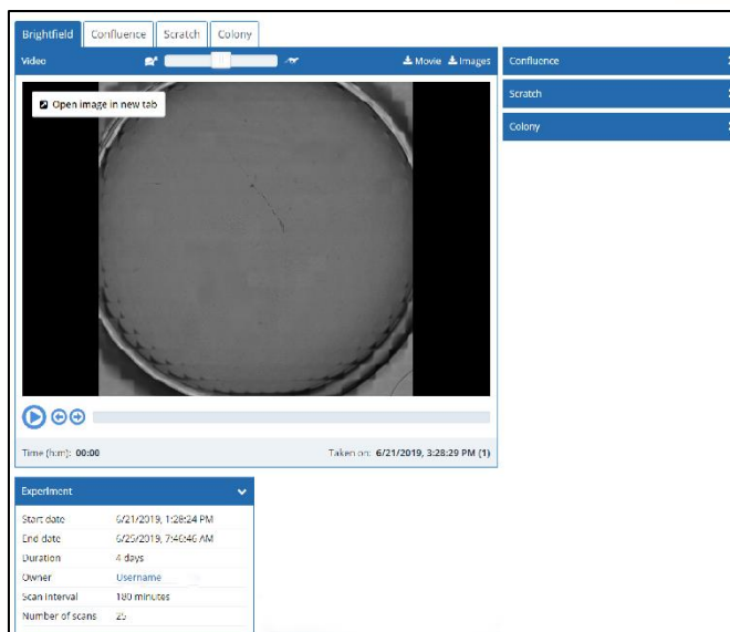
fig. 34. The Area page consists of a) time-lapse movie pane, b) graph pane(s) and c) experiment pane
